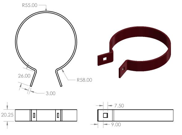
**Description**– Full range of Bolted Clip Head to suit Copper piping system includes extensions shanks and
